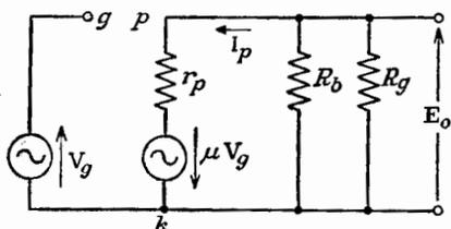
FIG. 7-13. Thévenin's circuit for the mid-frequency range.
