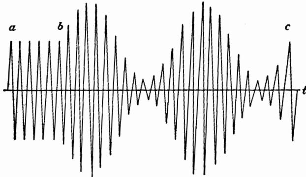
FIG. 5-1. Amplitude-modulated wave.
