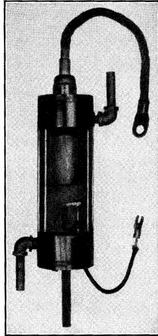
FIG. 13-12. Cutaway view of a water-cooled sealed-off ignitron.
