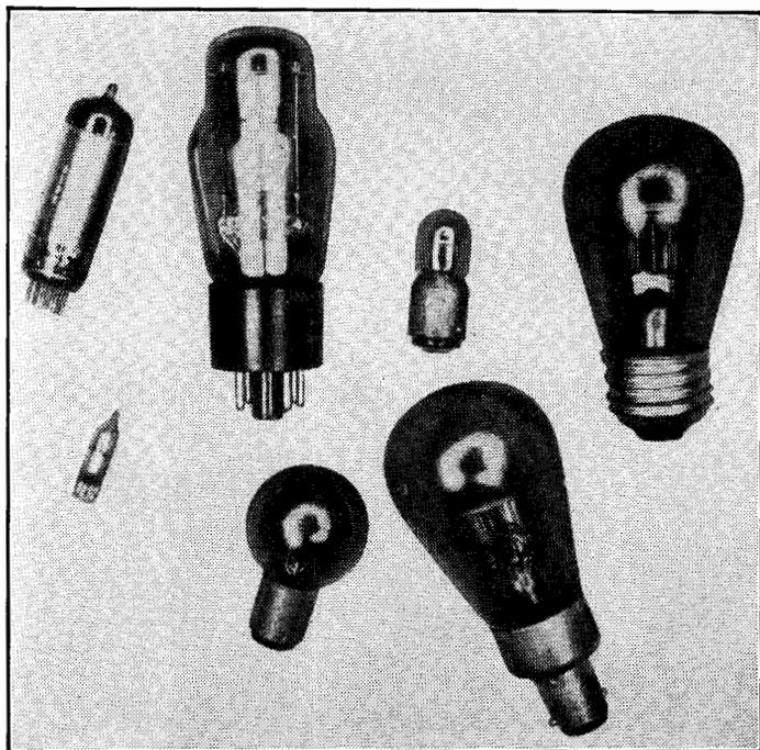
FIG. 13-5. Some common types of glow tubes.
