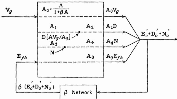
FIG. 10-5. A feedback amplifier with increased amplifier gain.
