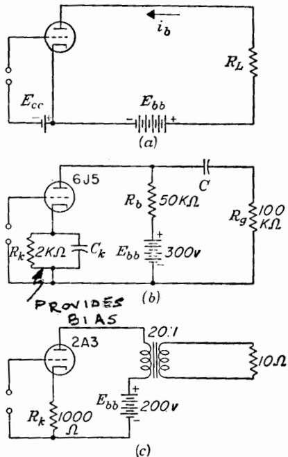
FIG. 6-3. Some common plate-load arrangements.
