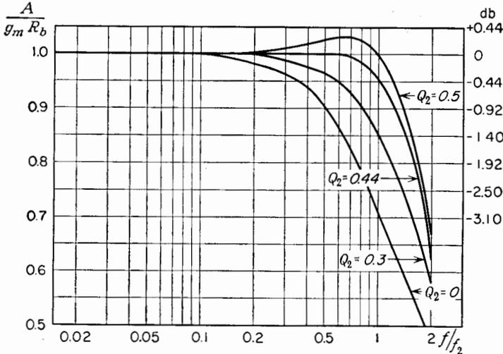
FIG. 7-37. Normalized curves of amplification vs. frequency.
