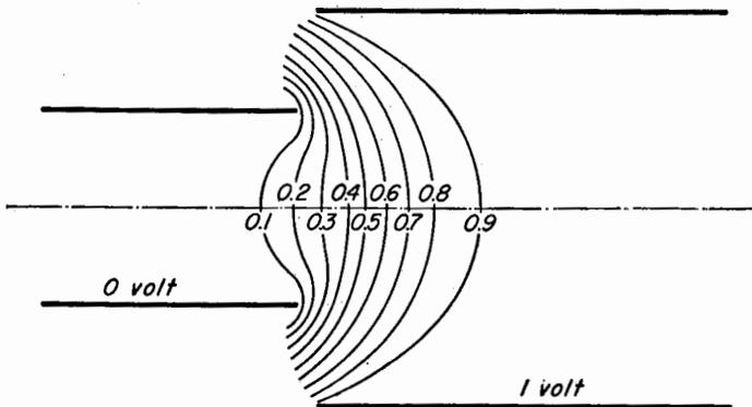
FIG. 1-15. Potential field of a two-cylinder electrostatic lens.
