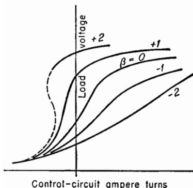
FIG. 16-26. Effects of negative and of positive feedback with magnetic amplifiers. ( $|\beta| \propto$  No. feedback turns.)
