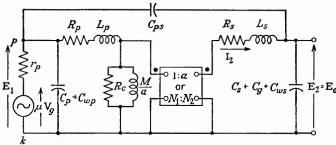
FIG. 7-67. An equivalent circuit for a transformer-coupled amplifier.
