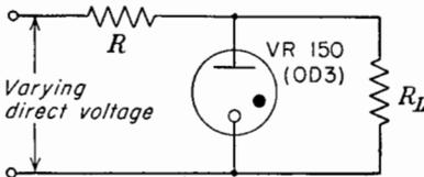
FIG. 13-6. Circuit for a voltage regulator using a V-R tube.
