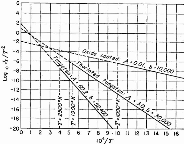
Fig. 2-4. Determination of constants in Richardson's equation.
