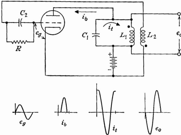
FIG. 5-20. A feedback oscillator.
