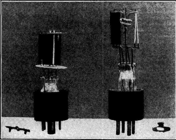
FIG. 3-1. Radio-receiver-type diodes.
