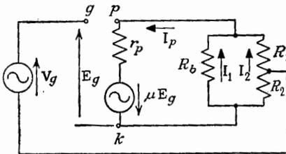
FIG. 6-25. Thévenin's equivalent for the circuit of Fig. 6-24.
