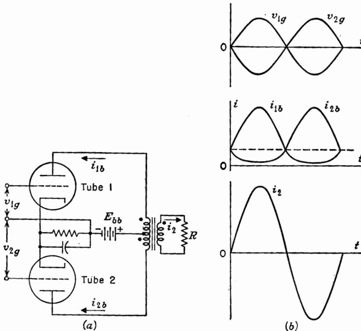
FIG. 5-17. (a) A push-pull amplifier. (b) Waveforms.
