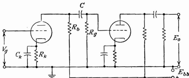
FIG. 7-10. An  $R$ - $C$ -coupled triode amplifier.
