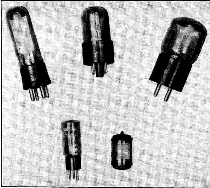
Fig. 15-5. Photoemissive cells.
