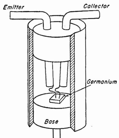
FIG. 16-13. Cutaway view of a transistor.
