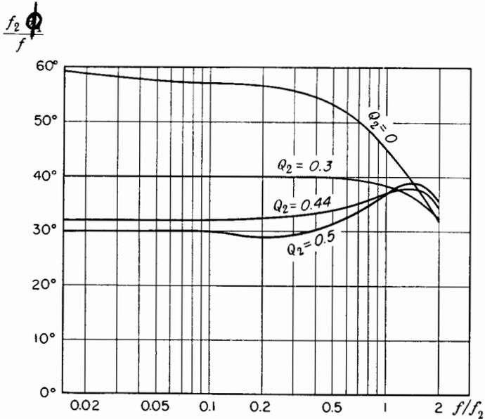
FIG. 7-39. Curves of phase shift vs. frequency.
