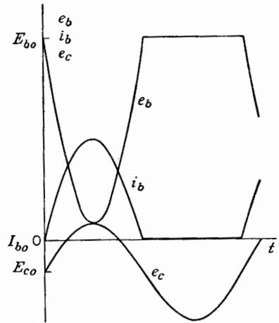
FIG. 8-4. Waveforms for class B operation.
