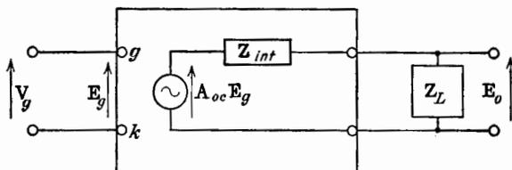
FIG. 10-8. A Thévenin's representation of a multistage amplifier.
