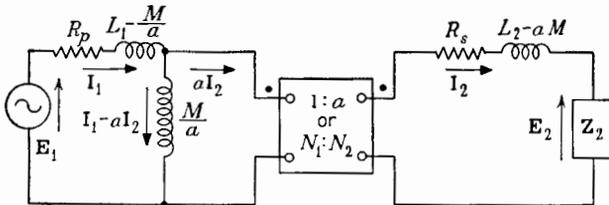
FIG. 7-62. Another equivalent circuit for a transformer.
