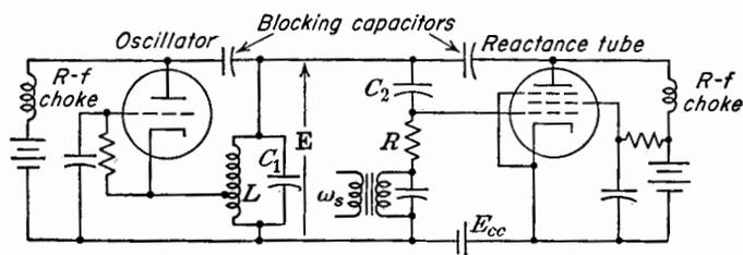
FIG. 12-23. A reactance tube modulating a Hartley oscillator.
