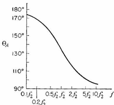
FIG. 7-25.  $\theta_A$  vs. frequency in the h-f range.
