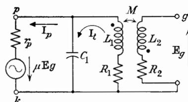
FIG. 11-10. Equivalent circuit for a tuned-plate oscillator.
