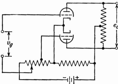
FIG. 7-9. A balanced voltage amplifier.
