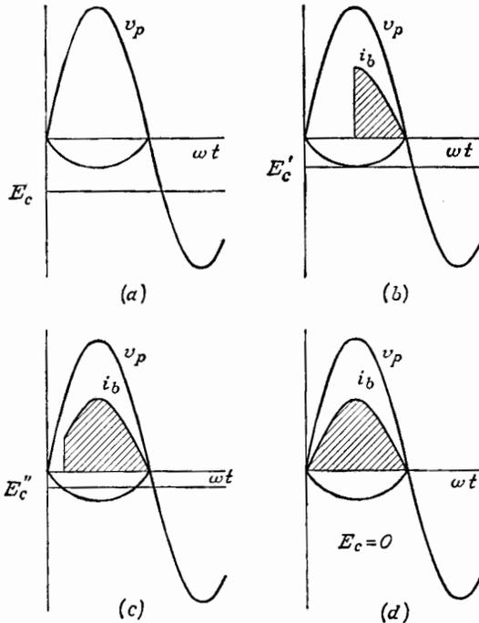
FIG. 14-24. Waveshapes illustrating d-c control of a thyatron.
