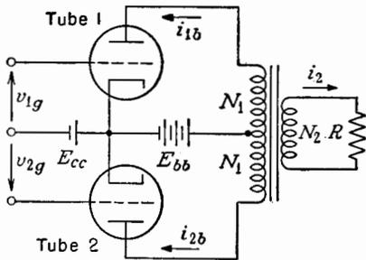
FIG. 8-17. A push-pull amplifier using fixed bias.
