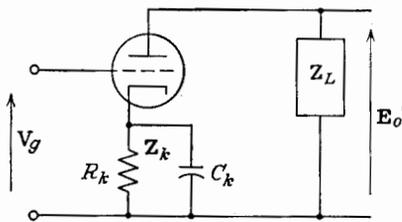
FIG. 10-16.  $R_k$  causes feedback if inadequately bypassed.
