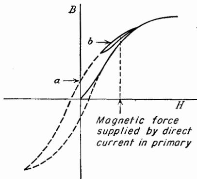
FIG. 7-66. Magnetic operation of a transformer.
