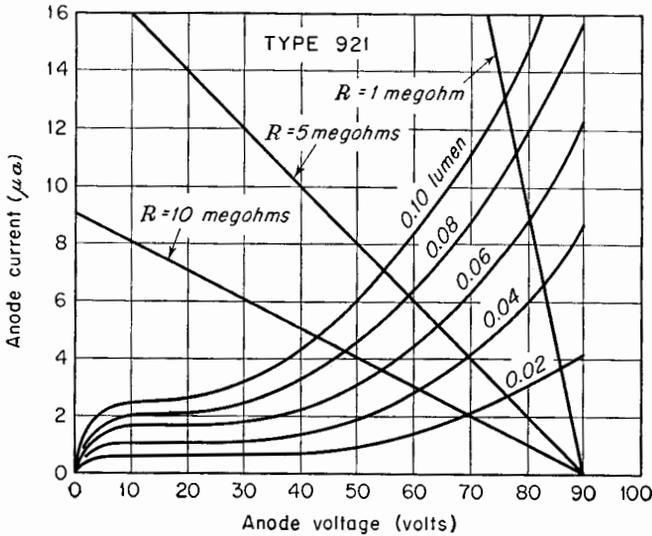
Fig. 15-8. Volt-ampere characteristic for a gas-type photocell.
