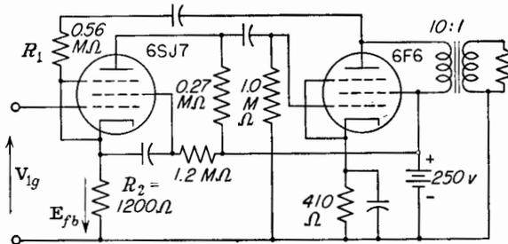
FIG. 10-20. A two-stage feedback circuit.
