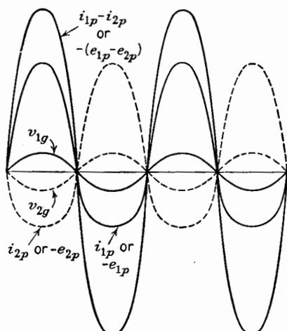
FIG. 7-46. Waveforms for the balanced amplifiers of Fig. 7-44.
