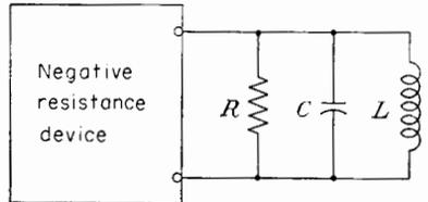
FIG. 11-15. Equivalent circuit for a negative-resistance oscillator.
