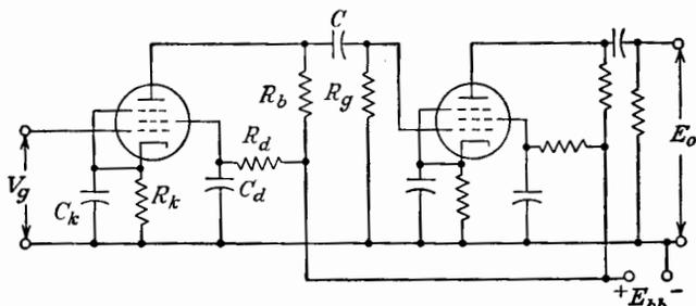
FIG. 7-11. An  $R$ - $C$ -coupled pentode amplifier.
