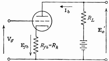
FIG. 10-7. An amplifier with simple current feedback.
