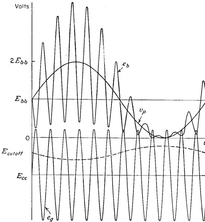
FIG. 12-7. Waveforms of grid voltage and of plate voltage with constant grid bias and 100 per cent plate-circuit modulation.
