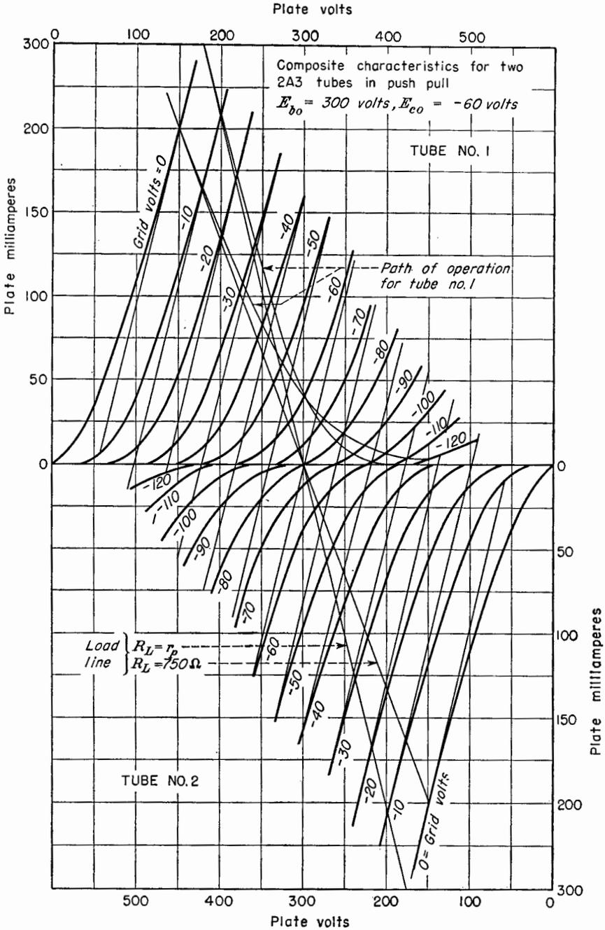
FIG. 8-21. Composite characteristics for two 2A3 tubes in class AB<sub>1</sub> push-pull.
