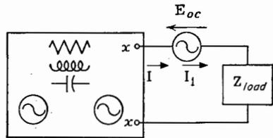
FIG. 6-15. (a) Linear bilateral network. (b) Thévenin's equivalent circuit.
