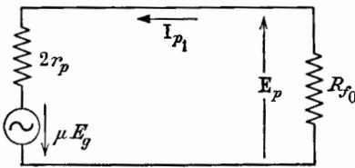
FIG. 9-8. An equivalent circuit useful for fundamental-frequency components.
