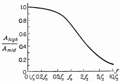
FIG. 7-24. Gain vs. frequency in the h-f range.
