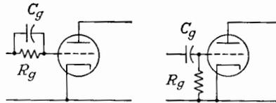
FIG. 9-12. Grid-leak-bias arrangements.
