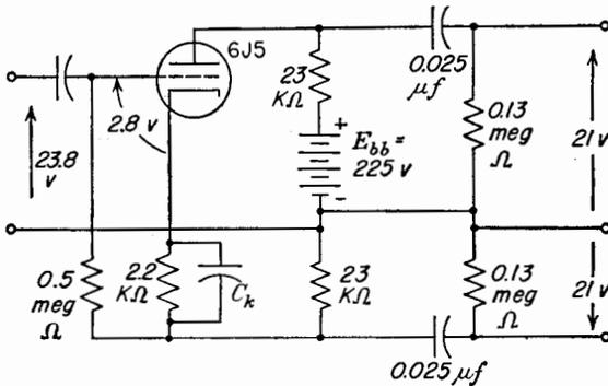
FIG. 7-49. A tube-manual design for a phase inverter.
