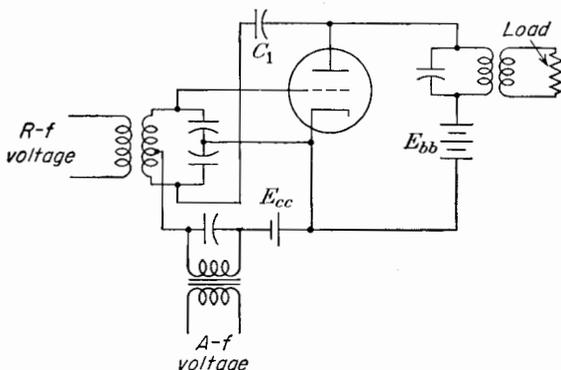
FIG. 12-9. A grid-bias-modulated class C amplifier.
