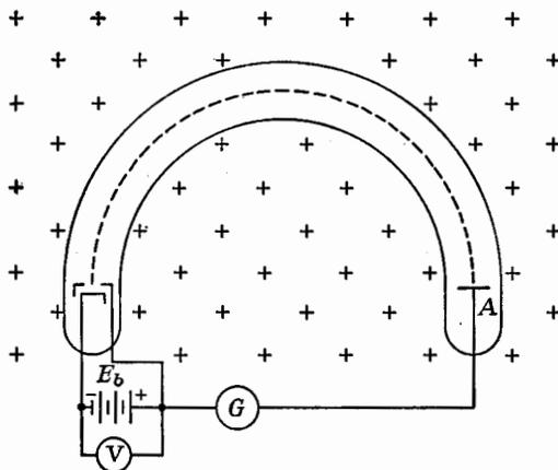
FIG. 1-10. Tube for measuring the charge-to-mass ratio for electrons.
