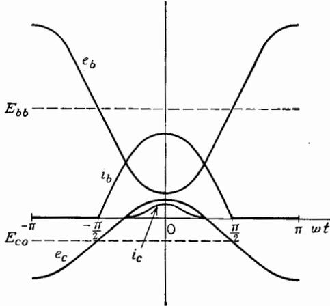
FIG. 9-2. Approximate waveforms for class B operation.
