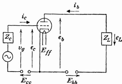
FIG. 6-1. A triode with a plate load.
