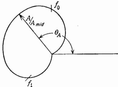
FIG. 7-73. Polar diagram for a transformer-coupled amplifier.  $Q_0 = 1$ .
