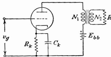
FIG. 5-14. A triode power amplifier.
