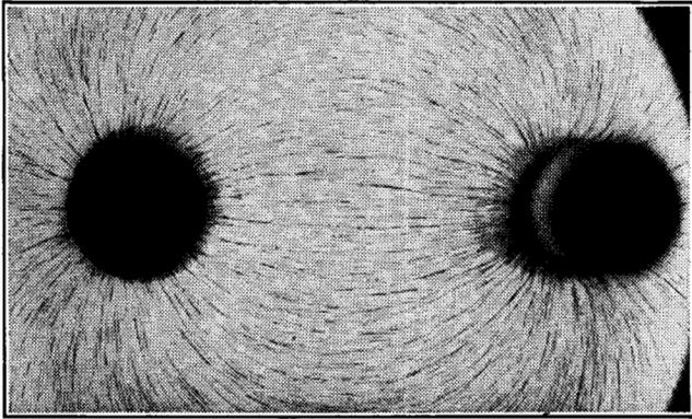
Fig. 1-5. Flux pattern between two parallel cylinders.
