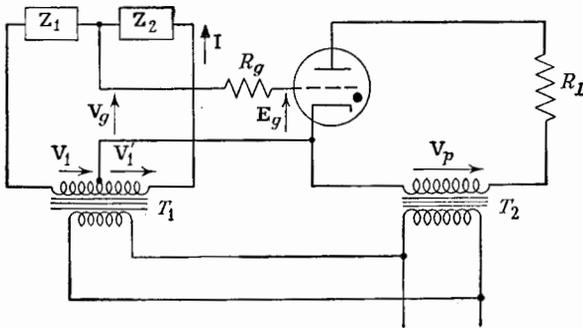
FIG. 14-27. A thyatron with phase-shift control.
