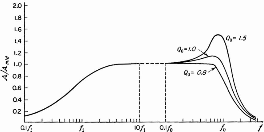
FIG. 7-71. Gain vs. frequency for a transformer-coupled amplifier.
