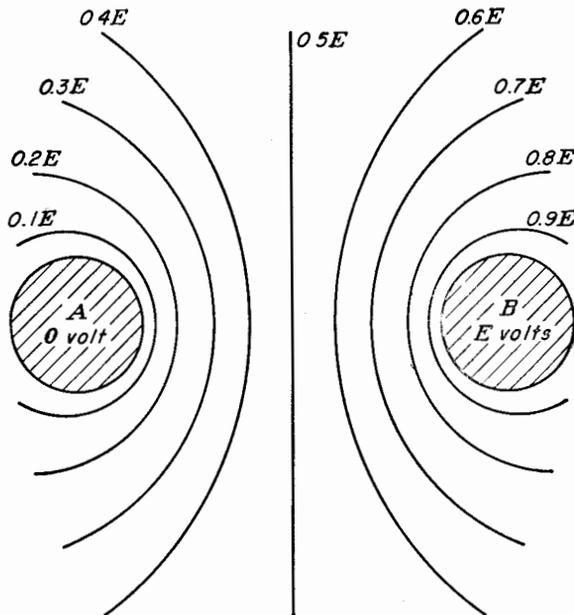
FIG. 1-3. The potential field between two parallel cylinders.
