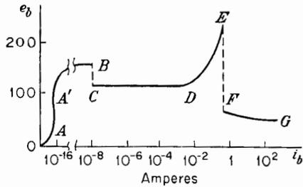
FIG. 13-2. Volt-ampere characteristics of a cold-cathode gas-discharge tube.
