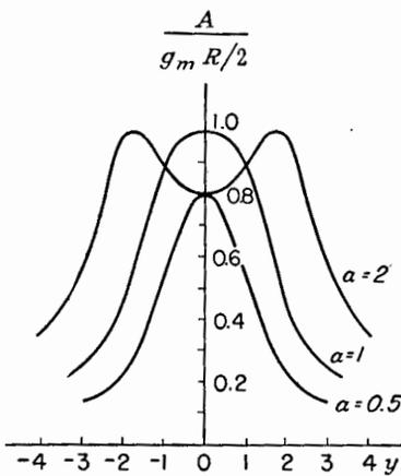
FIG. 7-85. Frequency response of a double-tuned amplifier.
