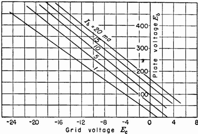
FIG. 4-6. Constant-current curves for a 6J5 triode.
