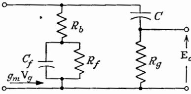
FIG. 7-43. Norton's equivalent of the circuit of Fig. 7-42.
