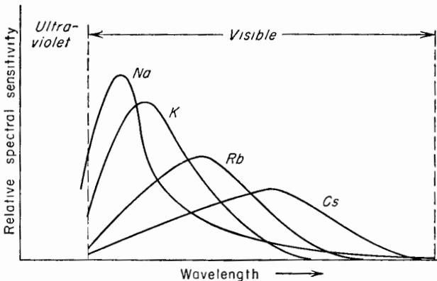
FIG. 15-3. Spectral-sensitivity curves for several pure metals.
