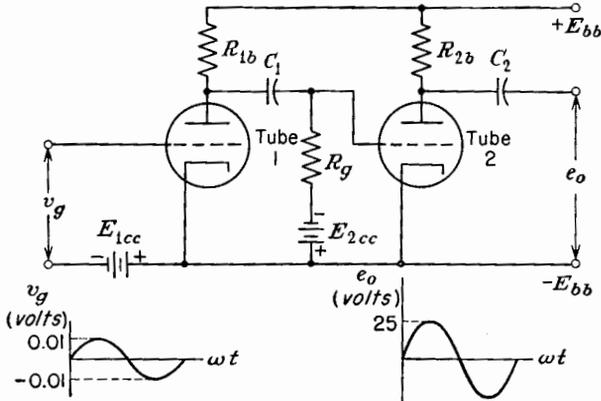
FIG. 5-10. A two-stage  $R$ - $C$ -coupled amplifier.
