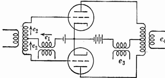
FIG. 12-12. Basic circuit for a balanced modulator.
