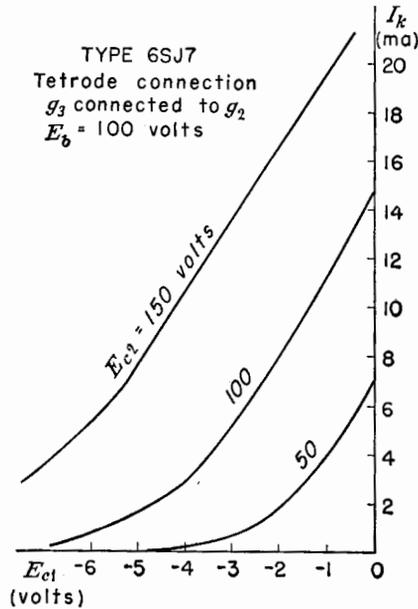
FIG. 4-19. Transfer characteristics for a tetrode—cathode current vs. grid voltage.
