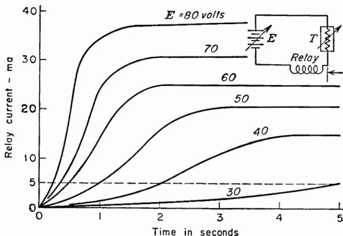
FIG. 16-6. Current vs. time curves for six values of the battery voltage in the circuit shown in the insert. (Courtesy of Bell Laboratories.<sup>3</sup>)
