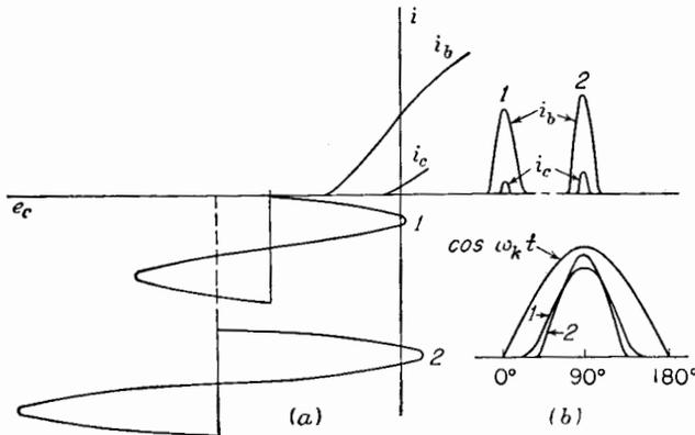
FIG. 12-30. Waveforms of  $e_c$ ,  $i_c$ , and  $i_b$  for the limiter.
