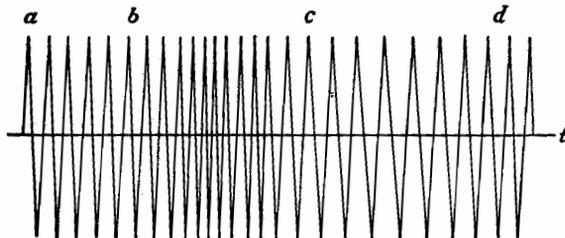
FIG. 5-2. Angle-modulated wave.
