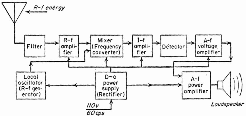
FIG. 5-4. Block diagram of a radio receiver.
