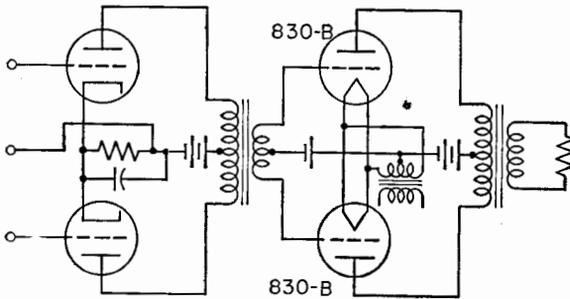
FIG. 8-24. A class B amplifier and its driver.
