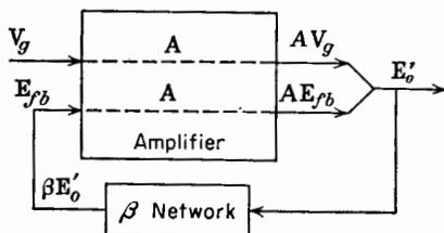
FIG. 10-2. Block-diagram representation of a feedback amplifier.
