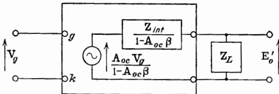
FIG. 10-11. A nonfeedback equivalent of a voltage-feedback amplifier.
