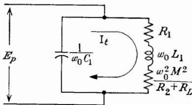
FIG. 9-6. The equivalent circuit for Fig. 9-5.
