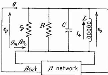
FIG. 11-2. The equivalent circuit for a regenerative-feedback oscillator.
