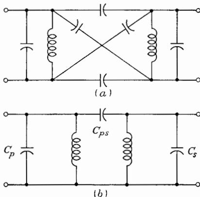
FIG. 7-63. Distributed capacitances in a transformer.
