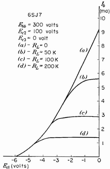
FIG. 4-25. Dynamic transfer characteristics for a 6SJ7 pentode.
