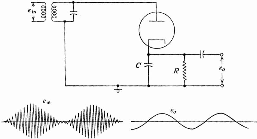
FIG. 5-7. A diode detector.
