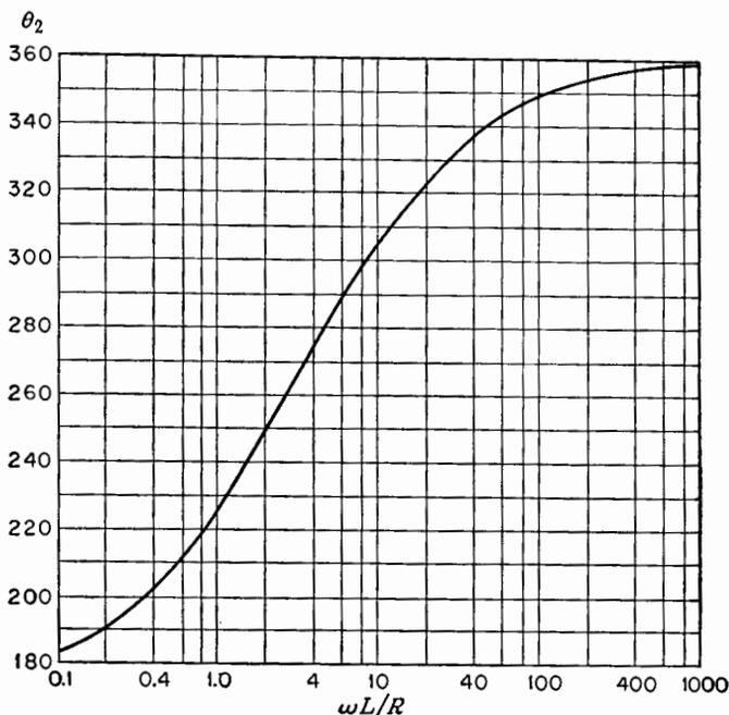
FIG. 14-17. Variation of extinction angle  $\theta_2$  with  $\omega L/R$  for a half-wave rectifier using a smoothing inductor.
