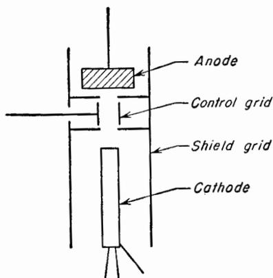
FIG. 13-16. Typical electrode structure for a shield-grid thyatron.
