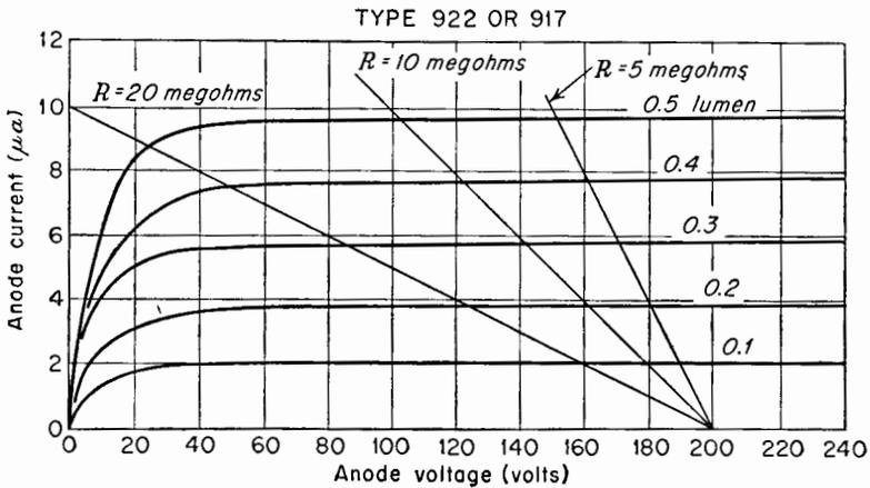
Fig. 15-6. Volt-ampere characteristic for a vacuum-type photocell.
