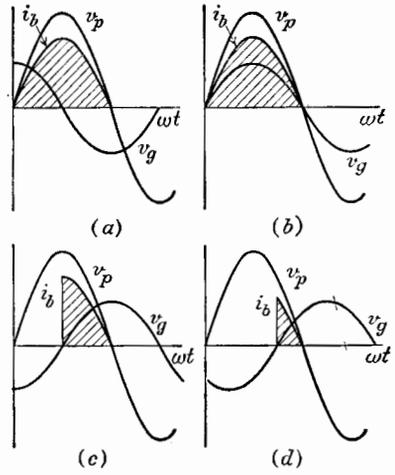
FIG. 14-26. Waveshapes illustrating phase-shift control.
