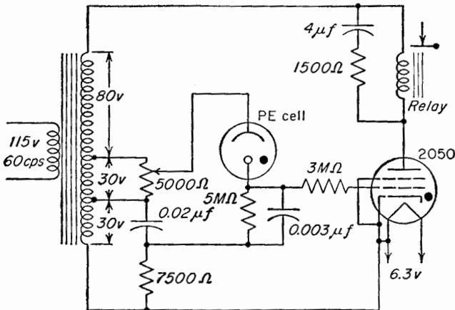
FIG. 15-12. Circuit diagram of the Westinghouse RQ Phototroller.
