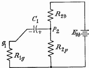
FIG. 11-26. Circuit applying to events just before tube 1 conducts.
