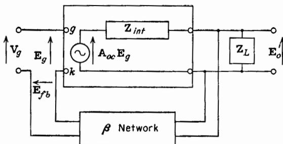
FIG. 10-9. A representation of a general voltage-feedback circuit.
