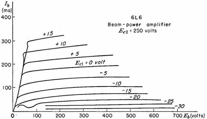
FIG. 4-30. Plate characteristics of a beam power tube.
