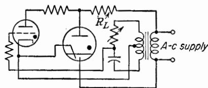
FIG. 14-33. Ignitron circuit using a thyatron for firing.
