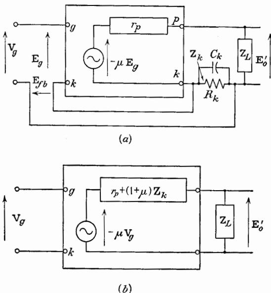
FIG. 10-17. Equivalent circuits for the amplifier of Fig. 10-16.
