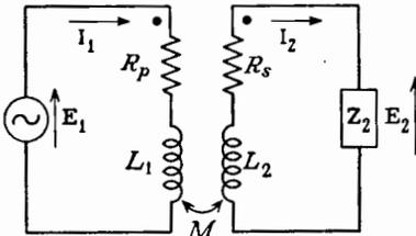
FIG. 7-61. An equivalent circuit for a transformer.
