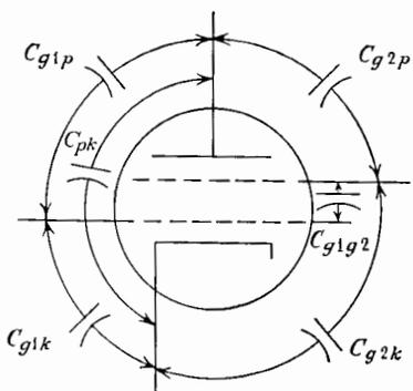
FIG. 4-15. Interelectrode capacitances in a tetrode.
